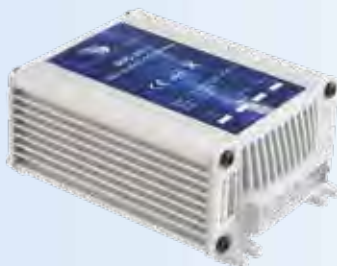
SR.202 Input V 20-35 Vdc - Output 13.6 Vdc Output: Amp. 20A - Eff. 90%
