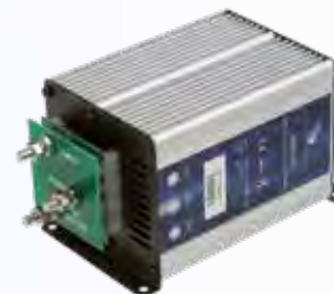
SR.210 Input V 20-35 Vdc - Output 13.6 Vdc Output: Amp. 60A - Eff. 90%
